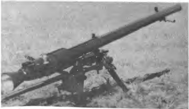
Figure 6-35. Recoilless anti-tank guns. Older weapons, such as the 82-mm B-10 (above, left) and the 107-mm B-11 (above, right), are now being replaced by the new 73-mm SPG-9 (below), which fires a rocket assisted projectile at ranges of about 1,000 meters.
